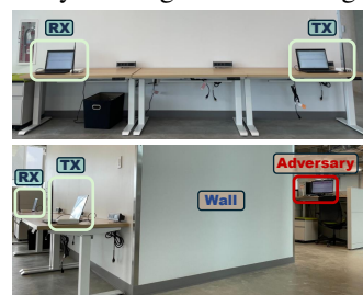
Fig. 20: Experiment Settings. A scenario where an adversary sends an adversarial signal from behind a wall in LoS Tx-Rx.
